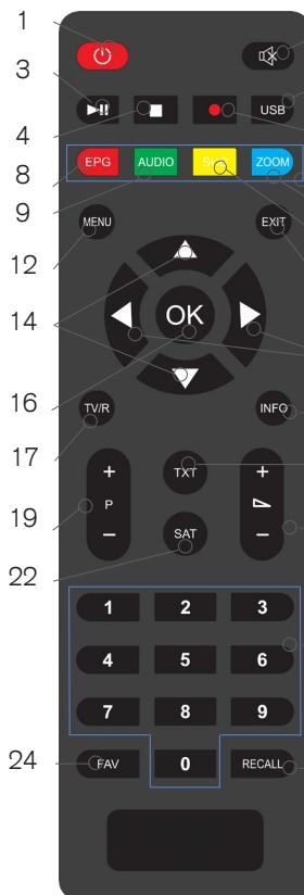
1. POWER: Switches receiver ON or in stand-by-mode.
