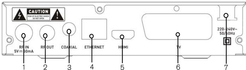
1. RF IN: Input of the digital tuner.
