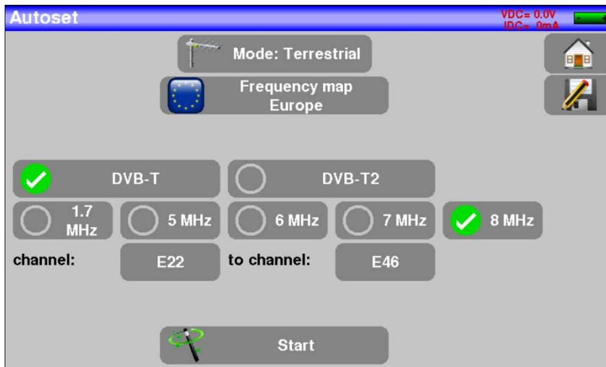
You can select the standards to be used (DVB-T, DVB-T2), the bandwidth, and the range of channels on which the search will be performed. The fewer options that are selected, the faster the results will appear.
