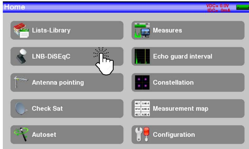
The following screen will be opened. If you need to power the satellite antenna make sure that the remote power is set to "ON". If it is not as in the image, press the icon where the satellite antenna is displayed and change the power to "ON".
