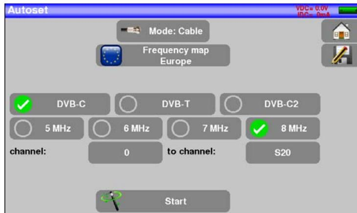
You can select the standards (DVB-C, DVB-T, DVB-C2), bandwidth, and channel range on which the search will be performed.
